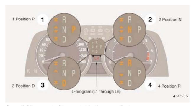
After switching on the ignition and starting the engine, the P or N positions and all of the arrows are indicated. In positions D or R, the single arrow for the shift direction to return to N is indicated (next to the N indicator).
